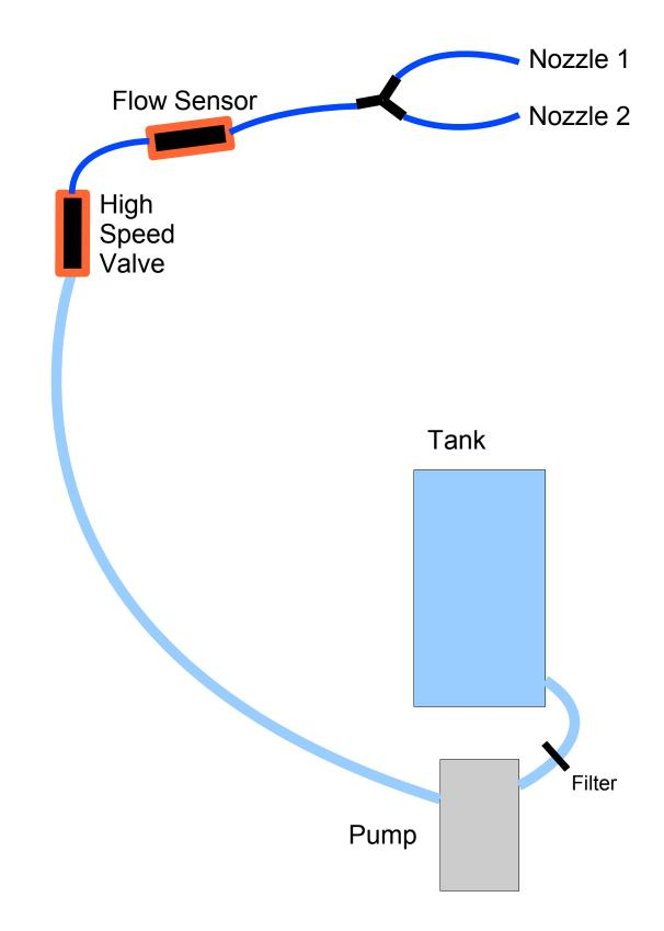
Hydramist water connections and water parts.
