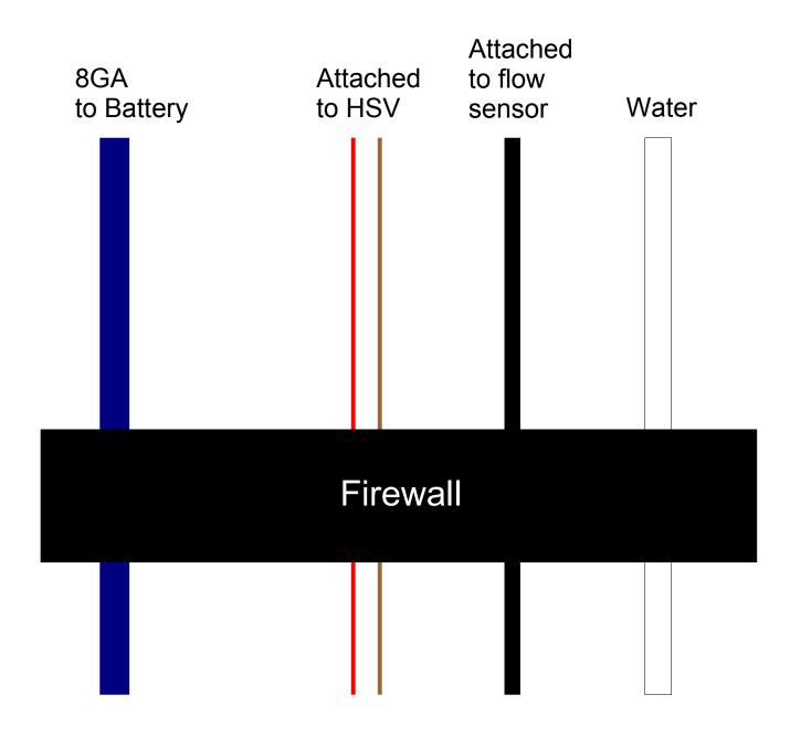
Hydramist items through firewall in standard setup with pump in the trunk. For a setup with the pump (and obviously tank) in the engine bay or front fender, the 8GA battery line and water tubing are obviously not going to go through the firewall.
